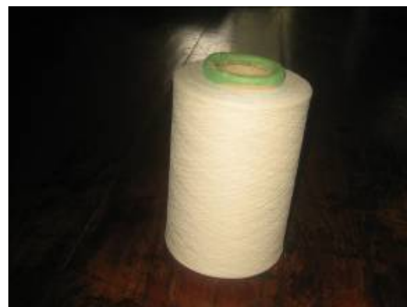
Fig. 4. Jute-cotton blended rotor yarn
