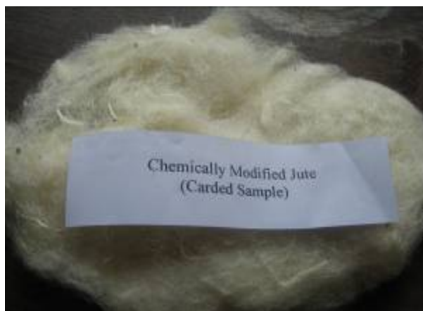
Fig. 3. Carded sample of modified jute fibers
