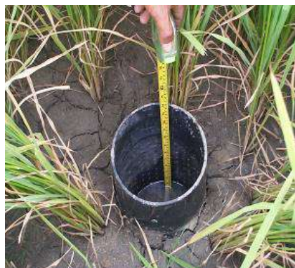
Plate 1. Water at 15 cm depth in porous tube
