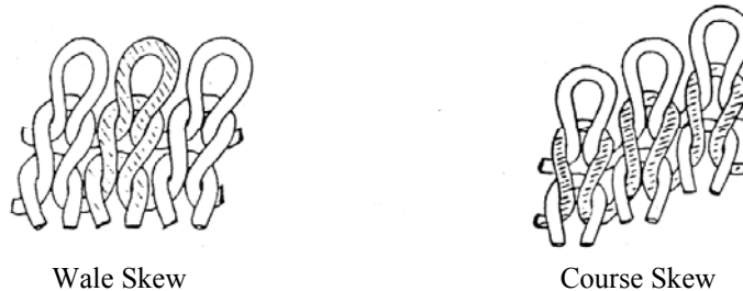
Fig. 1. Example of wale skew and course skew
