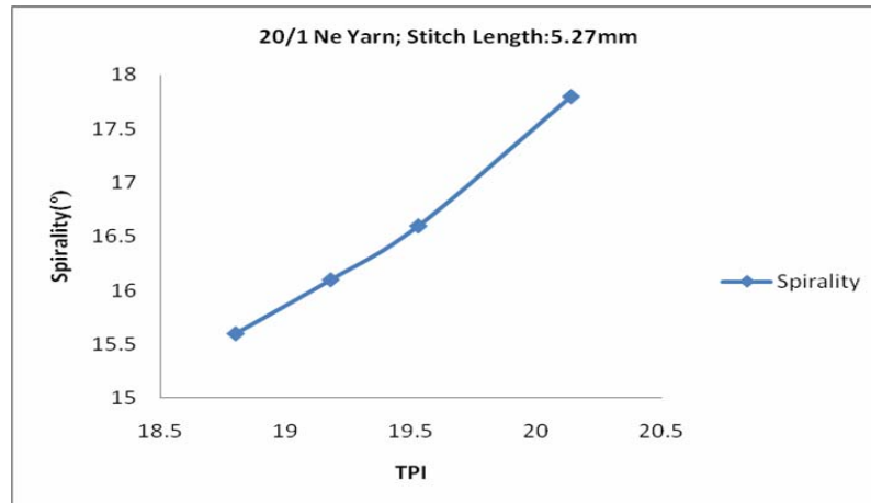
Fig. 4. Change of spirality due to variation of TPI in industrial relaxed state
