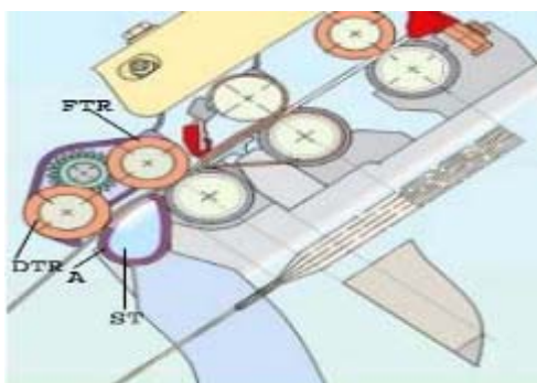
Fig. 4. Drafting equipment of the Suessen EliTe Compact system unit (ST-suction tube, A-lattice apron, FTR-front top roller, DTR-delivery top roller) (Frey 2001)
