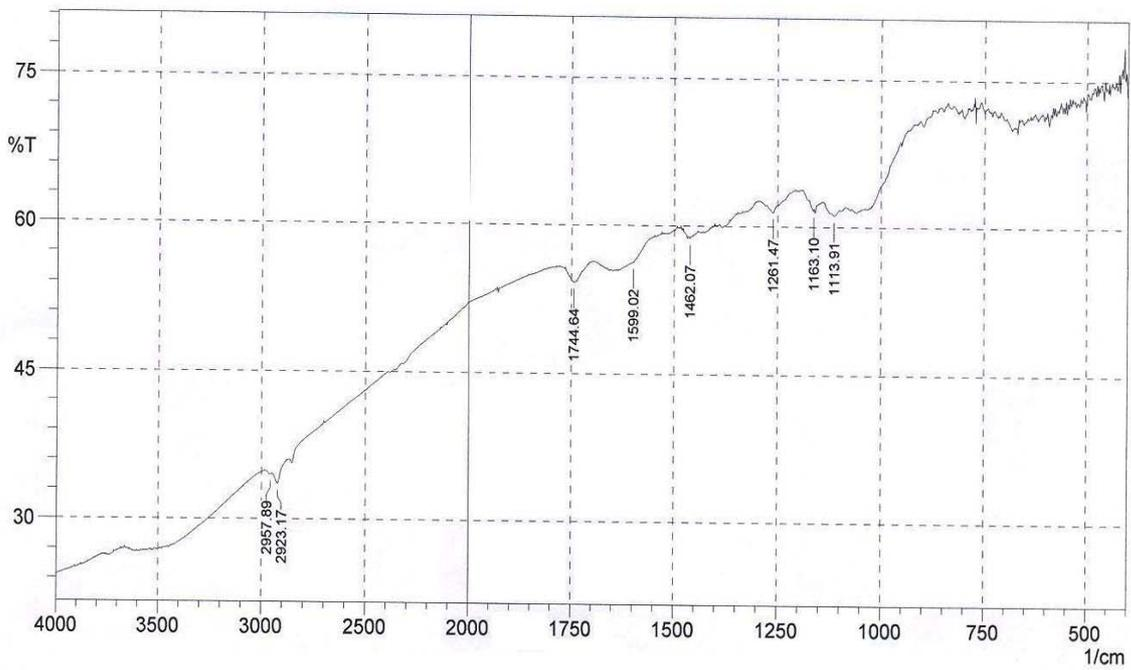
Figure 2. IR spectrum of existing (unmodified) yarn sample in KBr pellet
