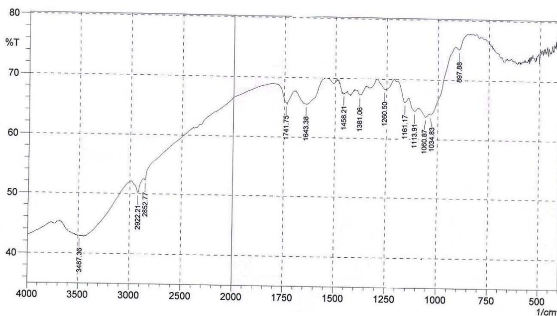
Figure 3. IR spectrum of existing (modified) yarn sample in KBr pellet
